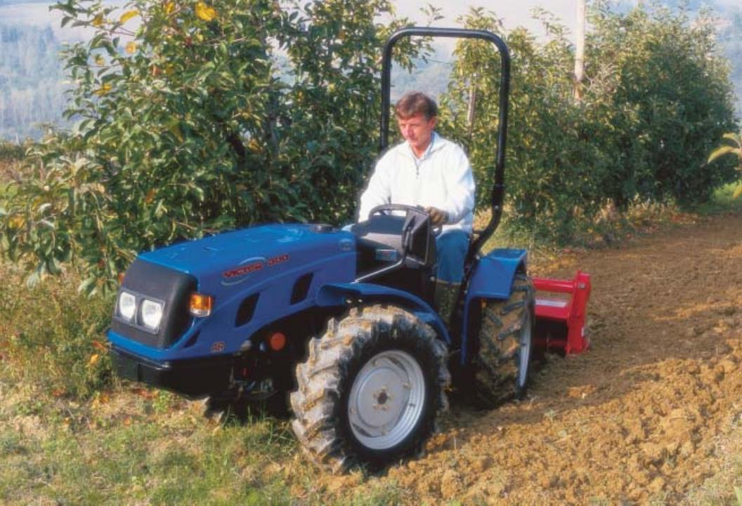
stipulated by even the most stringent standards (CARB, CE and EPA). By positioning all the main functions in the cylinder heads, we have managed to keep the overall dimensions of the engine block to a minimum. The **VICTOR 300** is equipped with a 1028 cc 3-cylinder engine that produces 19kW/26HP at 3400 rpm.
