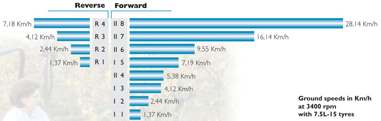
Ground speeds in Km/h at 3400 rpm with 7.5L-15 tyres
