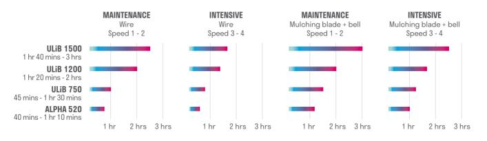
\* The battery life durations are calculated according to average power use observed during field tests. Tests carried out on sites of medium to high intensity.
