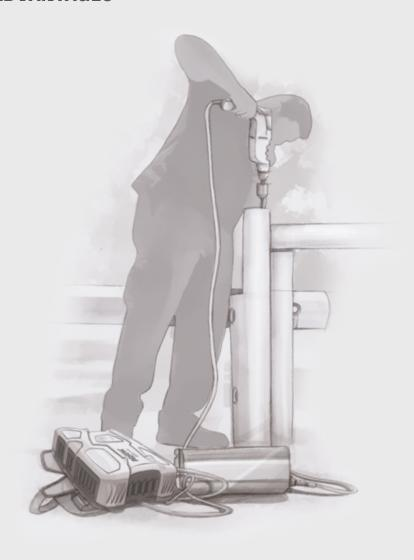
"The Power Converter converts the direct current from the battery into a maximum of 230 V/1,000W alternating current."
