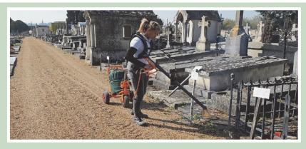
The Easy+ kit combines the mobile gas storage capacity with the mini thermal lance mounted on the ergonomic backpack allowing one hand to operate the lance and the other to position the trolley.
