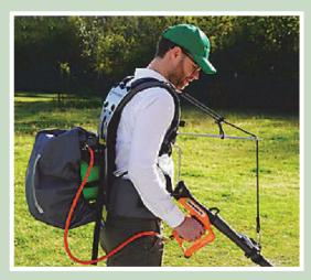
The thermal lance is supported by the harness allowing one hand operation with virtually zero effort. This kit weighs no more than a knapsack sprayer and may be used left or right handed. It is ideal for spot treatment and difficult to access situations. The nozzle may be rotated through 360° to tackle vegetation at different heights and angles.
