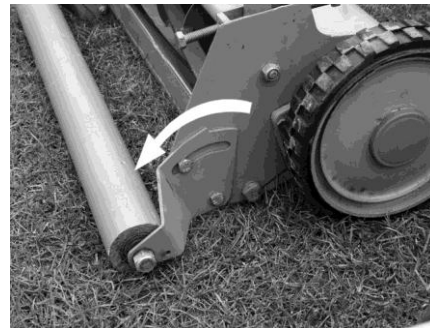
Fig. 7. Arrow shows highest [transport] position for roller.
