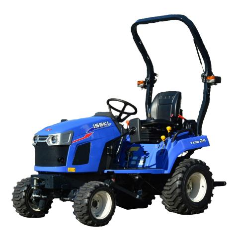
The new TXGS24 replaces the successful TXG237. It benefits from a flat easy-access platform, clear automotive style dashboard and controls, with switchable four-wheel drive makes the TXGS24 very user friendly. Individual forward and reverse pedals give the operator precise control.
