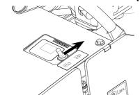
Prior to starting the machine, ensure that it is in transport mode and check that the transport lock is engaged.
