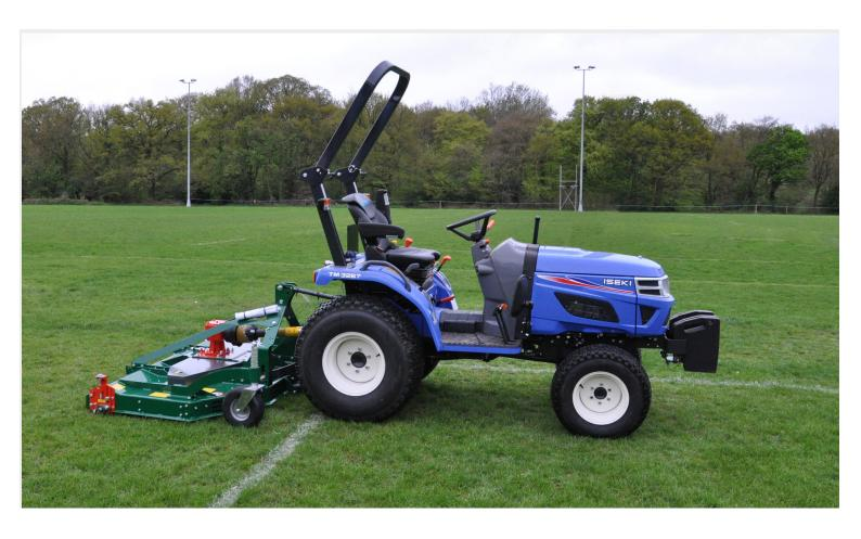
The new ISEKI TM3267 is a versatile 25hp diesel compact tractor with a three range hydrostatic transmission. The ISO-mounted operator's platform combined with ergonomically positioned controls ensures operator comfort during extended working periods. The 3-point linkage has a lift capacity of 600kg or 800kg (TM3267 only) when fitted with the high-capacity lift kit.
