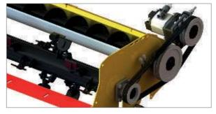
V-belt for reliable power transmission and overload protection.
