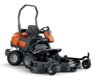
Powerful Hybrid commercial front mower. Two electric motors power the wheel drive axles, while the PTO and electric generator are powered by a 1123 cm<sup>3</sup> Kubota diesel engine.
