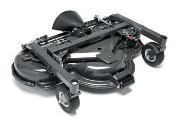
Commercial Combi decks offering both BioClip® (mulching) and rear ejection. The decks have a low profile heavy duty box frame and replaceable side skid wears. The shell has been stamped from a single piece of 4.5 mm thick piece of metal to optimise airflow, resulting in cutting high efficiency. Both deck sizes feature manual height adjustment.
