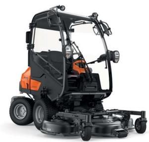
Highly productive large capacity diesel machine fitted with cabin for long shifts and all year use in very large areas.
