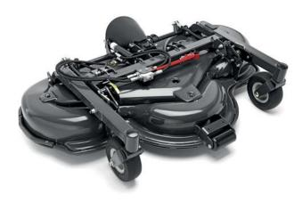
Commercial Combi decks offering both BioClip® (mulching) and rear ejection. The decks have a low profile heavy duty box frame and replaceable side skid wears. The shell has been stamped from a single piece of 4.5 mm thick piece of metal to optimise airflow, resulting in cutting high efficiency. Both deck sizes feature hydraulic height adjustment, adjustable from the seat.
