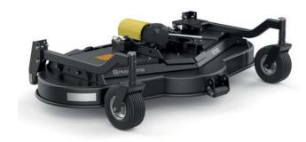
Professional, high-capacity rear discharge cutting deck. The R180 is a heavy-duty 180 cm cutting deck with rear discharge, for use with Husqvarna P 535HX. Designed for the professional user seeking a wide, high-performance cutting deck for efficient mowing of large areas and long dense grass. Shaft driven with bevel gear. Requires counterweight.
