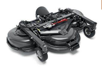
Commercial Combi decks offering both BioClip® (mulching) and rear ejection. The decks have a low profile heavy duty box frame and replaceable side skid wears. The shell has been stamped from a single piece of 4.5 mm thick piece of metal to optimise airflow, resulting in cutting high efficiency. Both deck sizes feature hydraulic height adjustment, adjustable from the seat. Hydraulic kit required when used with P 520D.
