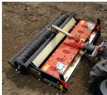
Working depth can be continuously adjusted using the manual spindle
