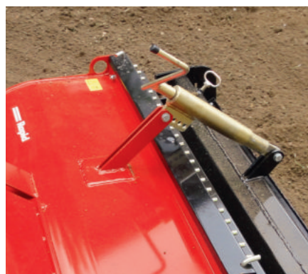
Manual spindle for continuously adjustable tilling depth
