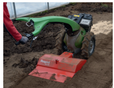
Laterally adjusted handlebar
