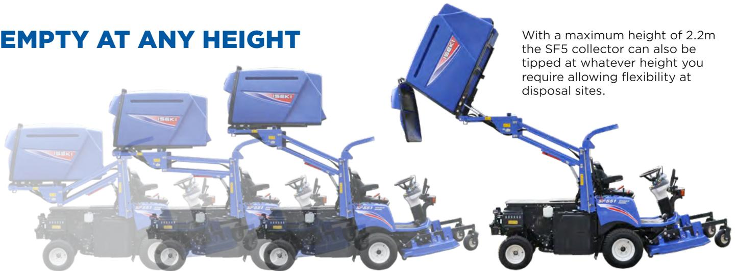
With a maximum height of 2.2m the SF51 collector can also be tipped at whatever height you require allowing flexibility at disposal sites.
