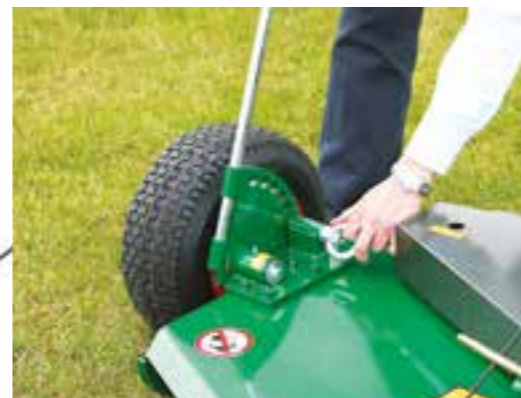
HEIGHT OF CUT IS SET BY REPOSITIONING THE WHEELS BY MEANS OF A SPRING LOADED PIN MECHANISM ON THE WHEEL BRACKETS
