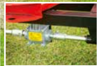
GROUND DRIVEN GEARBOX WITH SPINNER DISENGAGEMENT
