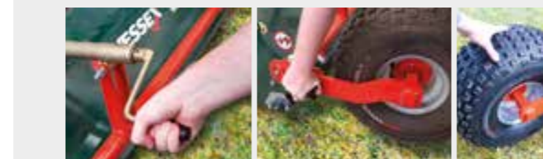
Step 1 RAISE WHEELS & REPOSITION HEIGHT ADJUSTER
