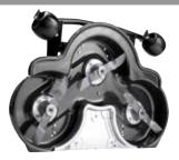
Combi cutting decks offer two cutting methods: BioClip® and rear ejection. As the deck is stamped from a single piece of metal, with no seams and sharp bends to trap cuttings, the result is market-leading mulching and super-efficient ejection. Fits to all 300 series models.
