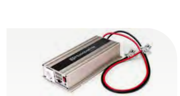
HUSQVARNA V1600F VOLTAGE CONVERTER Enables quick charging in the field by converting 12V DC from any lead-acid battery to 220 V AC for your QC500, QC330 or 40-C80 chargers. For professional or part-time use. 967 62 85-01
