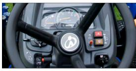
Easy to read electronically operated dashboard with rev counter, fuel gauge, PTO controls and light switches.
