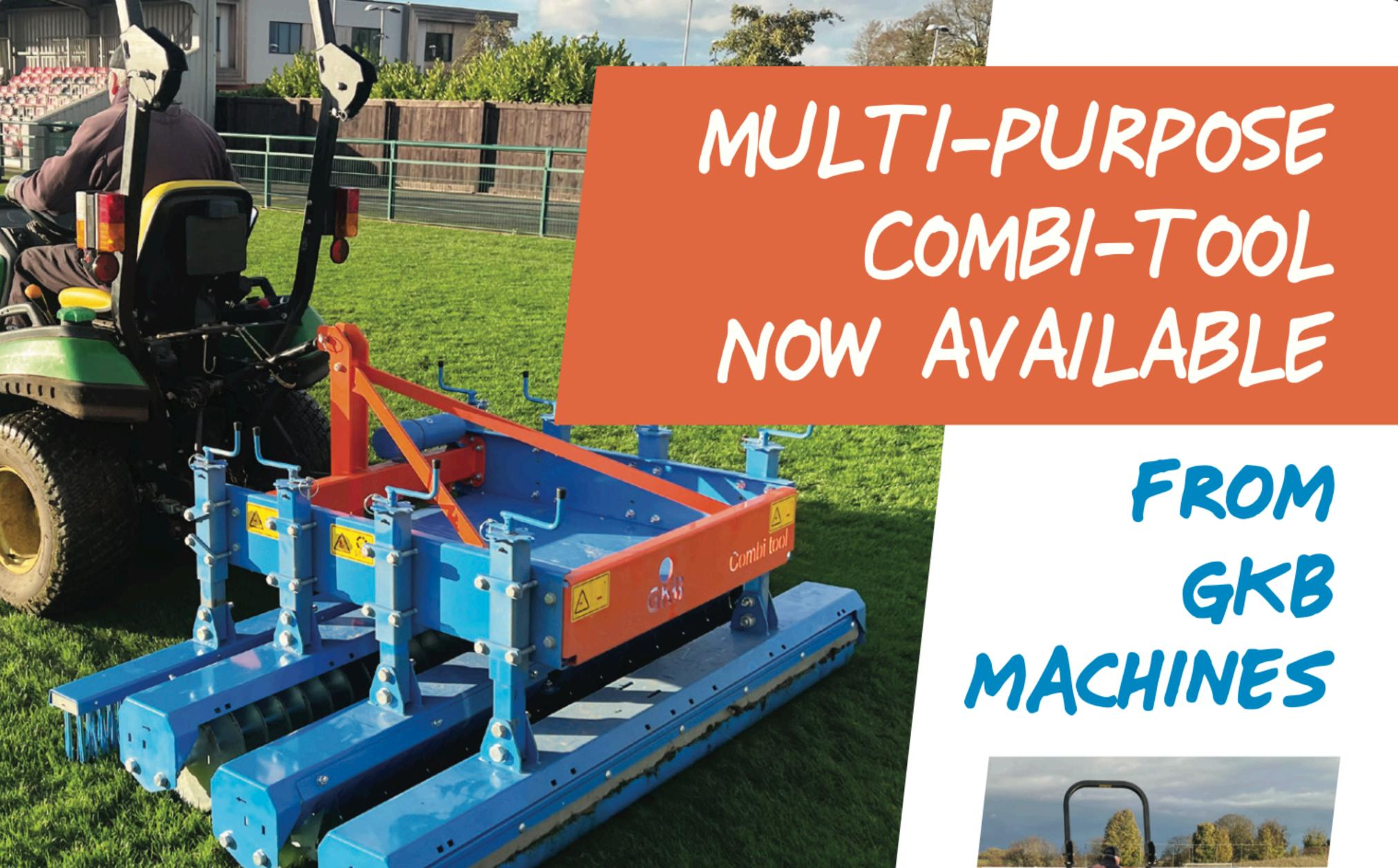
Combining versatility and value-for-money, GKB Machines have launched their new Combi-Tool. With a GKB engineered 3-point linkage frame and an ability to equip a range of maintenance attachments, the Combi-Tool gives turf managers the option of conducting multiple operations such as slitting, raking, rolling and brushing in one quick and simple pass.
