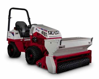
The EG520 Primary Seeder plants grass seed directly into bare soil with a consistent and accurate drop rate for perfect seed placement. With precise application adjustment and a removable calibration tray, easy adjustment for different grass seed types is possible.
