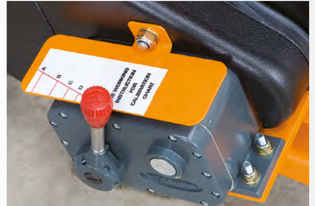
Zero Max Box for variable seed rates
