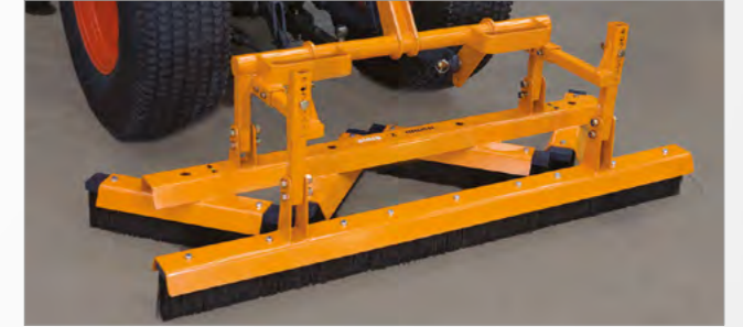
Twinplay frame suitable for 2 implements
