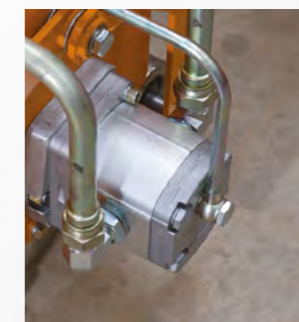
Direct Drive to reel shaft via hydraulic motor
