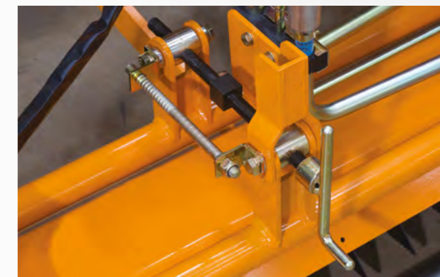
Micro adjusters for depth setting
