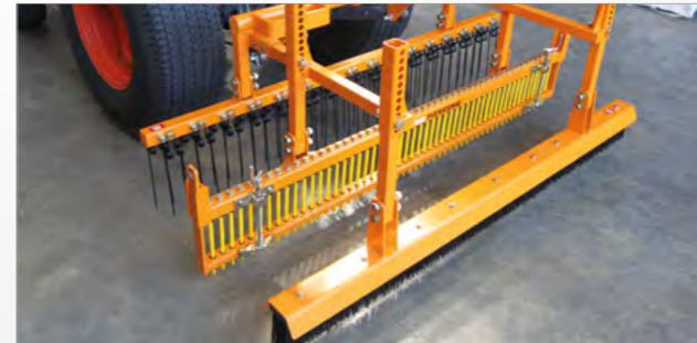
Tri-play frame suitable for 3 implements
