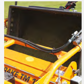
Large capacity collection box, shown with optional hydraulic tip kit
