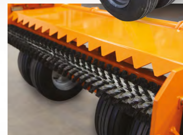
Close up of the rotating brush and oscillating plate
