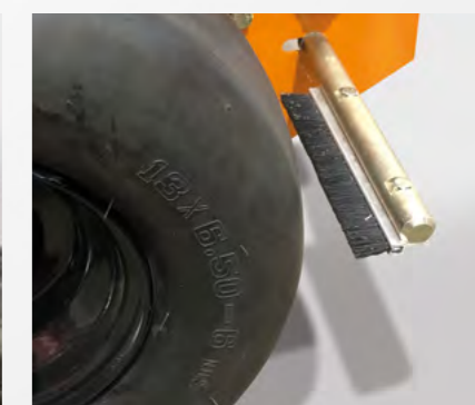
Slick tyres and debris removal brush
