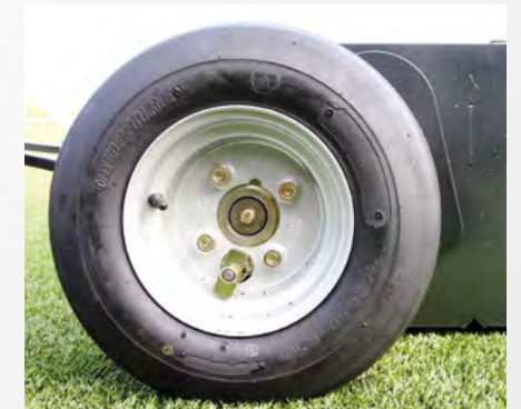
Simple “pull & twist” clutch levers on each wheel to disengage wheel drive to the brush during transport
