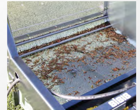
Debris collected and no infill
