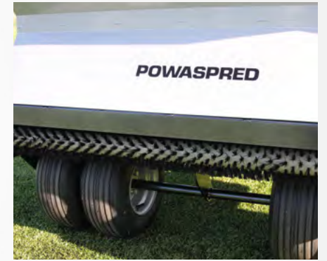
Rotating brush at point of discharge ensures even spread
