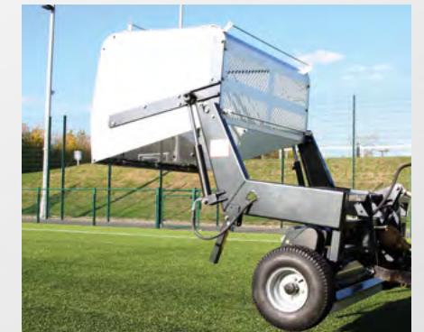
Hydraulic tip facility for easy emptying
