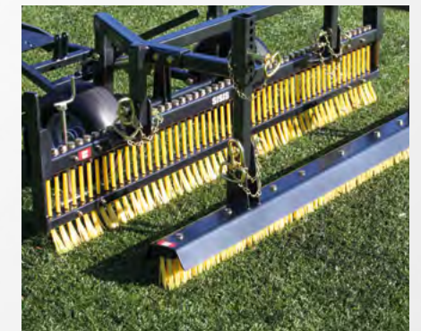
Towed frame with flexicomb and straight brush. The crossbar can be adjusted to shorten or lengthen the bristles for rubber crumb or sand infill
