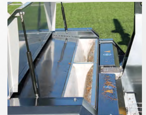
Easy to remove filter sections that contain fine dust particles
