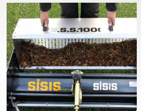
Easy-to-remove hopper and unwanted debris
