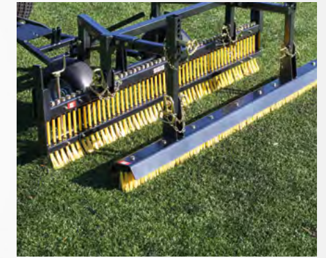
Flexicomb and brush combination ideal for rubber crumb or sand infill
