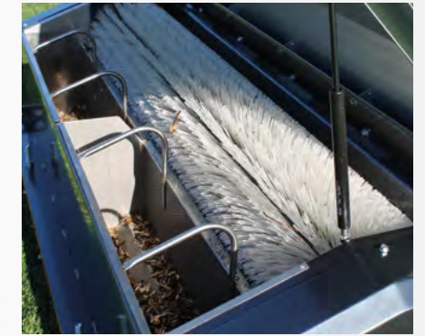
Removable sections with large debris
