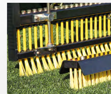
Softer bristles - Flexicomb crossbar set high for sand infill
