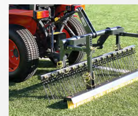
Twinplay with fine grooming rake and straight brush in action reducing compaction on rubber infill
