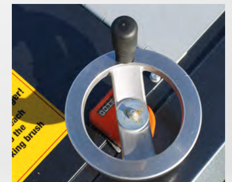
Easy to use hand wheel for working depth adjustment
