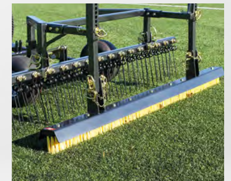
Towed frame with fine grooming rake and straight brush in action reducing compaction on rubber infill
