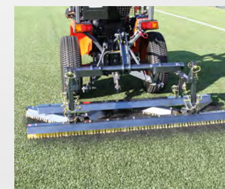
Zig Zag brush and straight brush combination at work on rubber crumb infill
