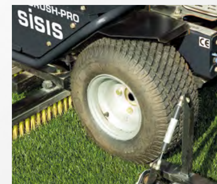
Treaded rear tyres with optional slick tyres
