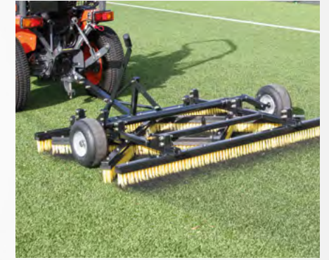
In action standing up the pile and moving the infill
