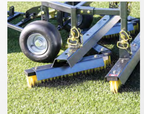
Zig Zag and brush combination ideal for rubber crumb or sand infill
