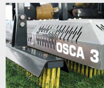
1.8m Straight Brush A straight brush added to the system will help to enhance the final finish
