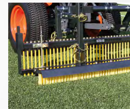
Adjustable crossbar on flexicomb alters length of bristles to meet the needs of rubber crumb or sand infill
