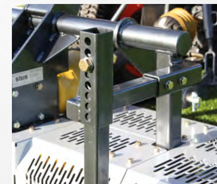
Twin play extension arms Twin play extension arms allow a 1.8m straight brush to be added to the system
