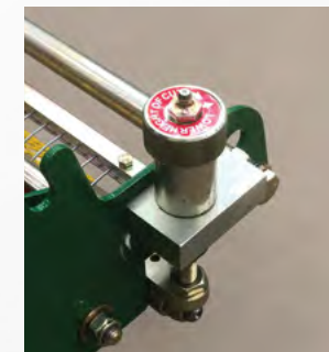
Simple tool free height of operation adjustment
