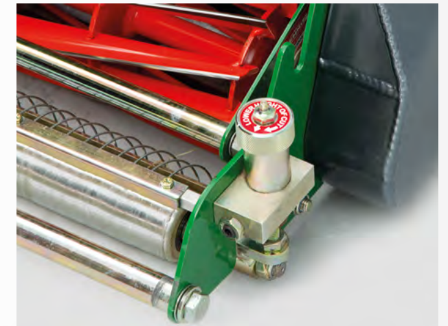
Simple 'without tools' click height adjustment in 0.25mm increments
