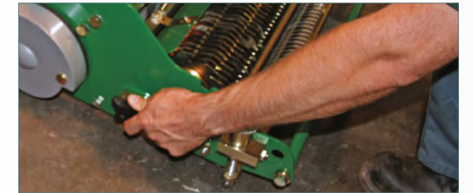
Loosen retaining bolt and slide cassette across
