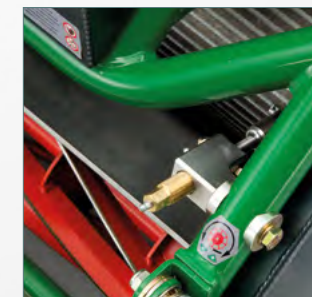
Easy adjustment of bottom blade to cylinder
