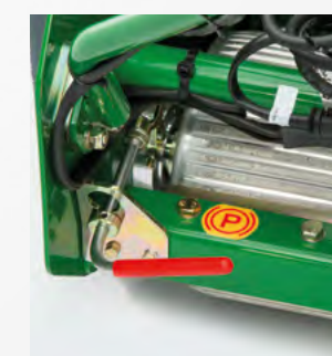
Simple lever operated mechanical parking brake
