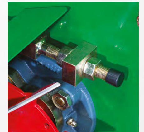
Adjustment of cylinder to bottom blade with a single spanner
