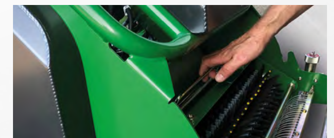
Lower cassette onto back tie bar and slide cassette across
