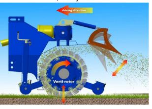
By means of our patented roller pendulum system, you can easily control the operating depth. As a unique bonus, we have provided the scarifying machine with a hydraulic adjustable cover. This is ideal when you are required to scarify near the edges and corners of a pitch.
