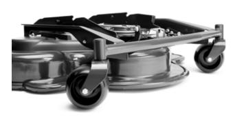
Husqvarna Combi decks combine very efficient BioClip mulching with rear discharge. The durable design is stamped from one piece, which contributes to its high efficiency, thanks to the optimised airflow. X-models cutting decks come with electric height adjustment. Must be combined with Power outlet kit.
