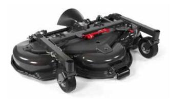
Husqvarna Combi decks combine very efficient BioClip mulching with rear discharge. The heavy-duty design is stamped from one piece of 4.5mm steel, which contributes to its high efficiency, thanks to the optimised airflow. Shaft PTO driven. All decks are equipped with replaceable side skid wears
