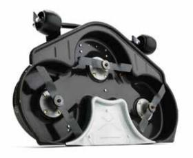
Husqvarna Combi decks combine very efficient BioClip mulching with rear discharge. The durable design is stamped from one piece, which contributes to its high efficiency, thanks to the optimised airflow.
