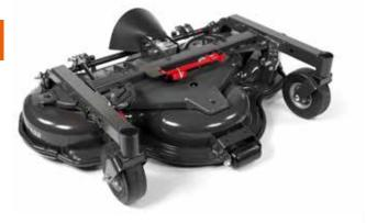
Husqvarna Combi decks combine very efficient BioClip mulching with rear discharge. The heavy-duty design is stamped from one piece of 4.5mm steel, which contributes to its high efficiency, thanks to the optimised airflow. Shaft PTO driven. All decks are equipped with replaceable side skid wears
