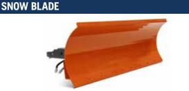
Rugged steel snow blade. Hydraulic adjustment and 140cm working width. Requires counterweight & hydraulic kit (P 520D). Requires support wheels and rubber scraper.
