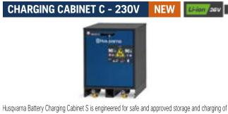
lithium-ion batteries. This 230V under-bench cabinet can easily be placed under worktops due to its low height and offers 90 minutes of fire resistance from the outside in and from the inside out\*.
